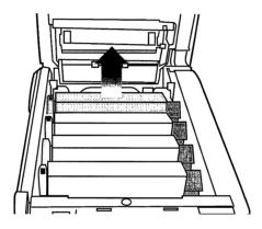
**5.** Put the cartridge down gently onto a piece of paper to prevent toner from marking your furniture and to avoid damaging the green drum surface.
