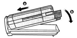
**10.** Push the coloured release lever (1) away from you to lock the toner cartridge onto the new image drum unit and release toner into it.
