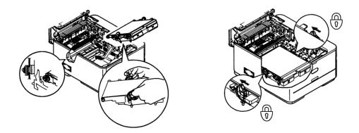
**8.** Push the locking levers towards the rear of the machine. This will secure the belt unit in place.
