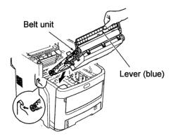
(3) Rotate the two blue lock levers in the direction of the arrow (9), and confirm that the belt unit is secure.
