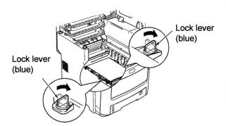
(4) Return the four image drum cartridges to the machine.
