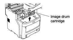
(2) Cover the image drum cartridges with paper to minimize their exposure to light.
